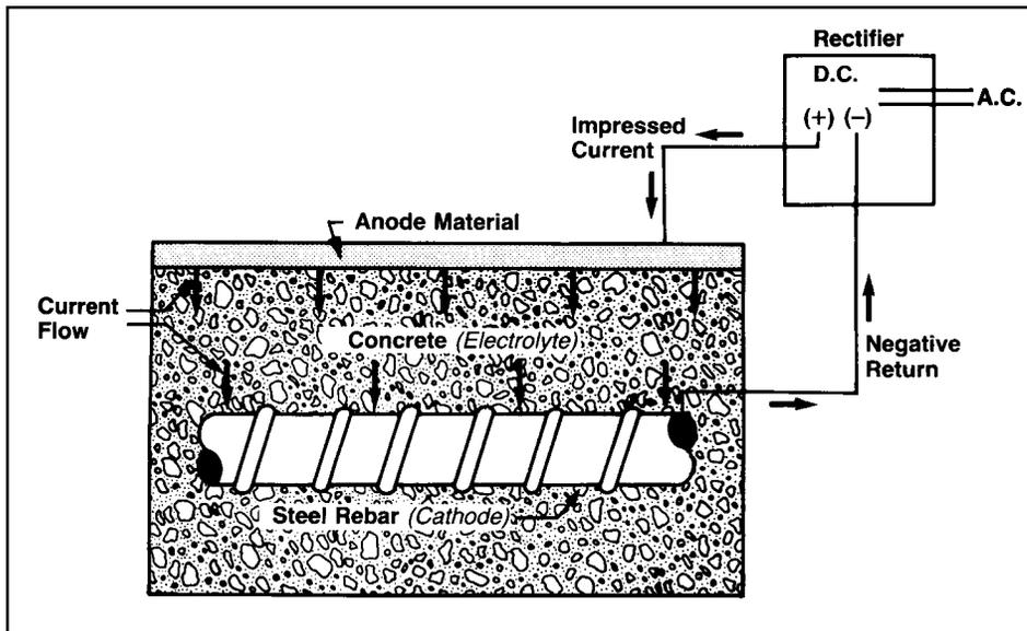
Figure 2. Basic layout required for cathodic protection. (Diagram: Report No. FHWA-DP-34-3 12/88)
