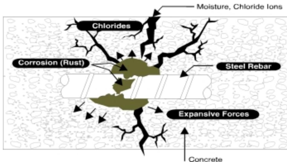
Figure 1. Schematic of concrete deterioration due to corrosion. (Diagram: Report No. FHWA-DP-34-3 12/88)
